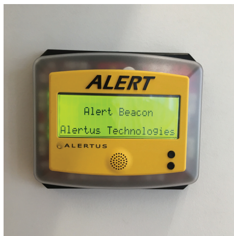
This is the alert beacon students will hopefully notice in buildings around campus. It is pictured in its normal, inactive state, but will blink red in the event of an emergency.
